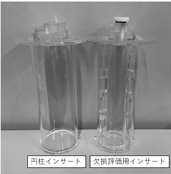
Fig. 1 Photos of defect insert and cylindrical insert.
