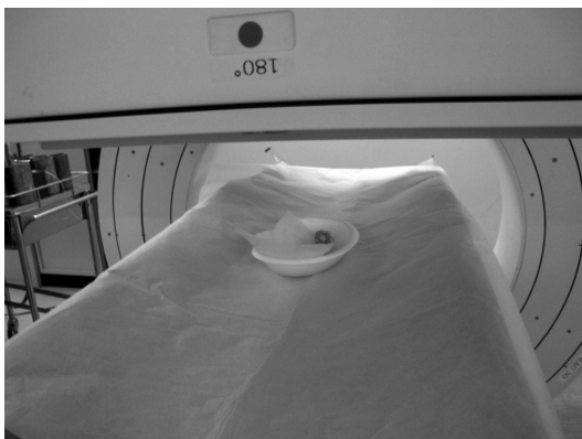
Fig. 2 Geometric arrangement of the syringe measurement シリンジ測定の幾何学的配置
